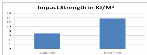
**Fig 6.** Impact strength of Sisal/Glass fibre composites
