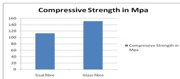
**Fig 4.** Compressive strength of Sisal/Glass fibre composites
