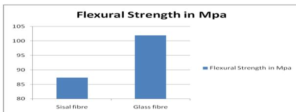
**Fig 5.** Flexural strength of Sisal/Glass fibre composites
