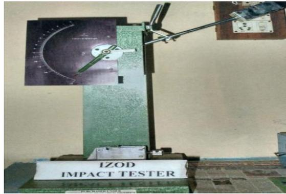
**Fig 2.** Izod Impact testing machine.
